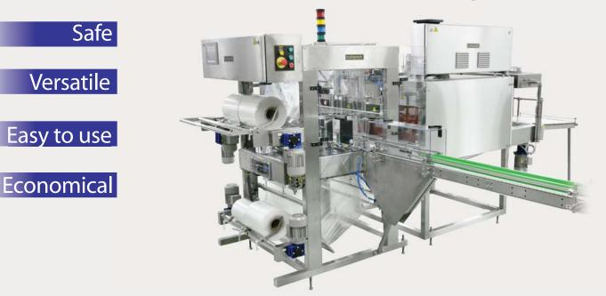
Autopack SLA with welding bar is an intermittent bundle shrink wrapper with side infeed and automatic grouping system. Specifically designed to handle brick type of packages from 125ml up to 1L, whether ESL gable top or UHT, the machine is available in single track or tandem configuration, grouping system by pneumatic or motor driven cycling pusher.
